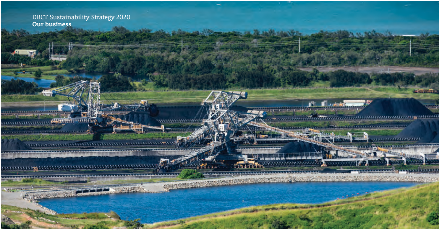
Stacker and stacker-reclaimer machines at work in the stockyard, with one of the on-site water storage facilities in the foreground.
